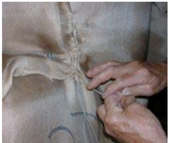
#42: Final stitching on 2D joints.
