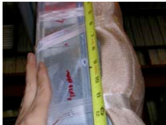
#24: Tape wrapped 6" o.c.
