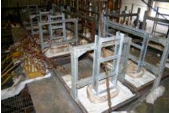
#85: Unexposed surface of test assembly.
