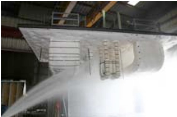
#107: Hose stream test.
