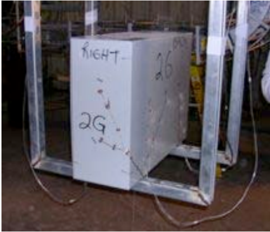
#55: Thermocouples on junction box.
