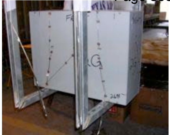
#56: Thermocouples on junction box.
