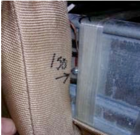
#27: 2C thermocouple at joint.
