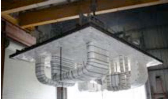
#105: Specimen ready for hose stream test.
