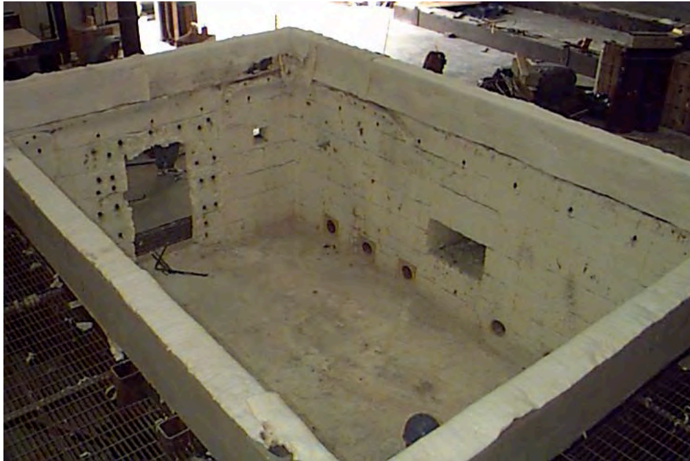
12' x 18' Horizontal Furnace (Overhead View)
