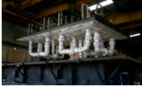
#98: Lifting specimen from furnace.
