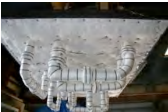
#113: Specimen ready for hose stream.
