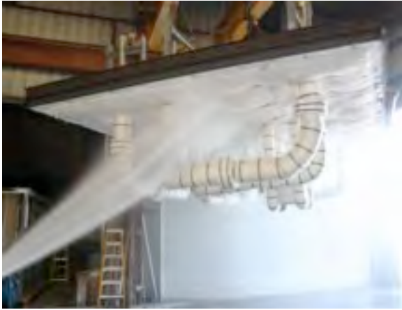
#115: Hose stream test.
