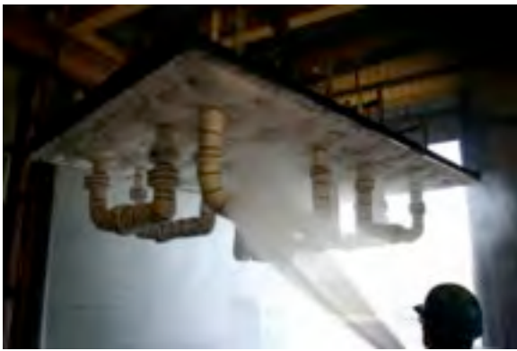
#117: Hose stream test.
