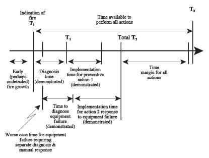
Figure C.3-2. Initial fire detection and multiple action (one action dependent on a separate diagnosis of an undesired equipment failure) with a single overall time margin and T<sub>3</sub>
