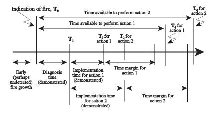
Figure C.3-4. Initial fire detection and multiple actions illustrating the application of multiple time margins and T<sub>2</sub>'s
