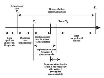
Figure C.3-3. Initial fire detection and multiple actions (one action dependent on completion of a prior action) with a single overall time margin and  $\mathsf{T}_3$
