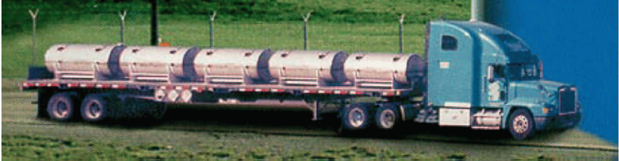
Figure C.1. Trailer carrying five UF 6 cylinders in overpacks (Photo courtesy of United States Enrichment Corporation [USEC 1999]).
