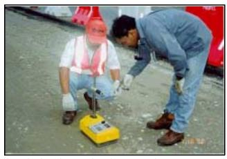
A typical moisture-density gauge in use.
