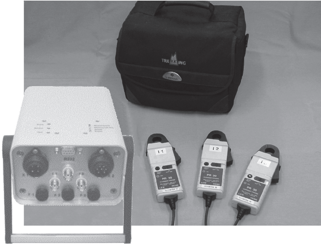
Figure 5: Pocket SIPLUG® with current clamps and transportation case
