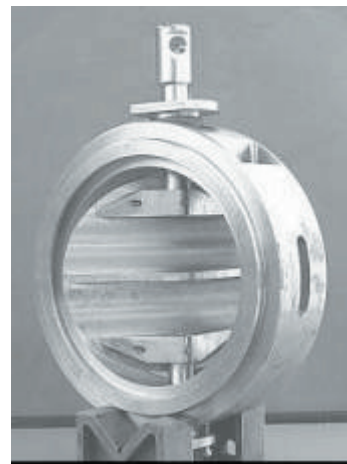
Figure 9: Triple-offset discs with large second offset were included in the test matrix.
