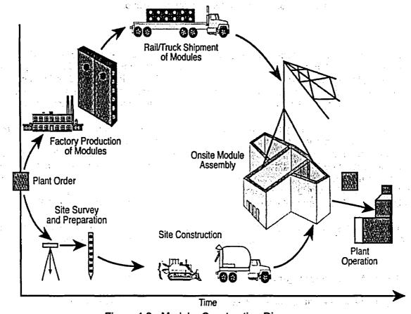
Figure 1.2 - Modular Construction Diagram
