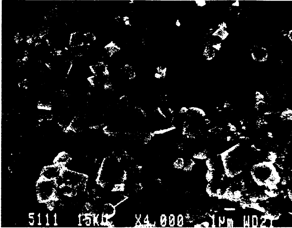
Figure 19. Electron micrograph of the surface of a Phase I Stellite 6 specimen after 19 days exposure to high-pH conditions; the large, zirconium-rich crystals are conspicuous.
