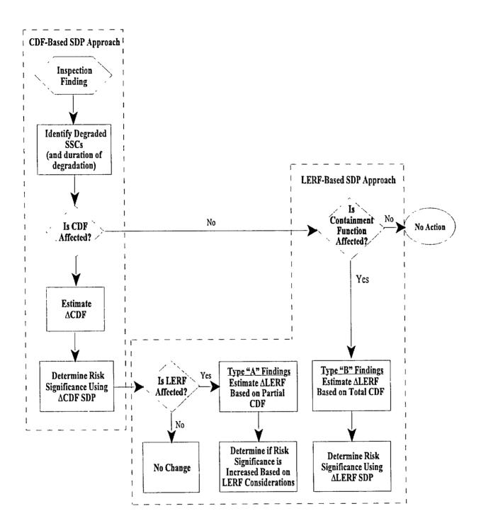
Figure 2.1 LERF-Based Significance Determination Process
