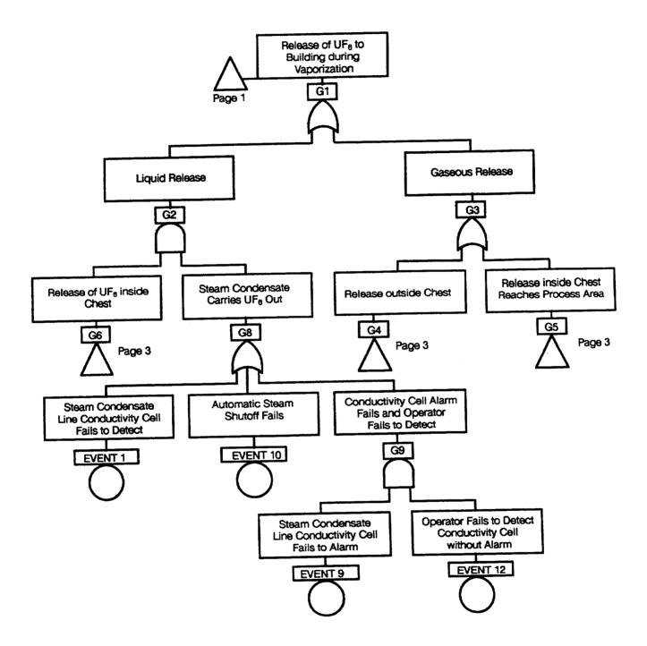
Fault Tree for Release of UF<sub>6</sub> During Vaporization (Cont.)
