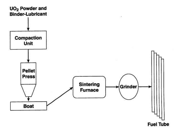
Figure B.1. Uranium Fuel Fabrication
