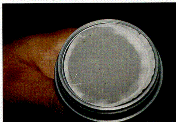
Figure 9. Smoke was filtered from smoke chamber to determine the smoke density.
