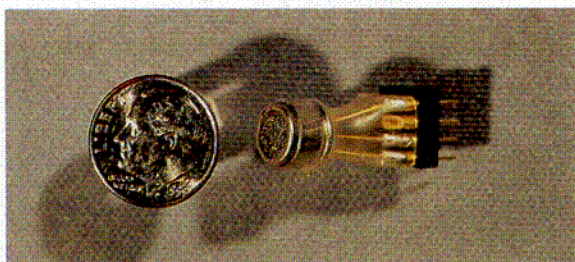
Figure 11. Humidity/temperature gage included in the smoke exposure chamber.
