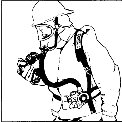
Figure 4-16. Open-circuit, pressure-demand SCBA.
