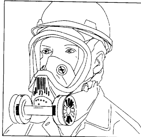
Figure 4-8. Full-facepiece with replaceable, cheek-mounted filters.
