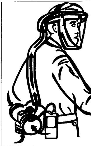
Figure 4-2. Loose-fitting facepiece with a powered air-purifying device.
