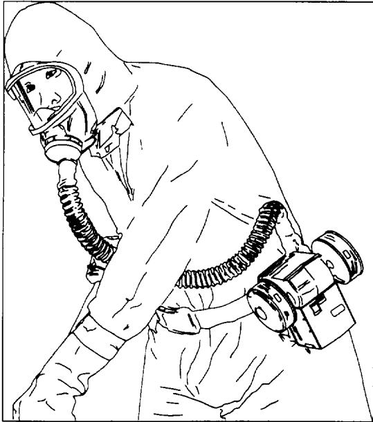
Figure 4-10. Powered air-purifying respirator with full facepiece.
