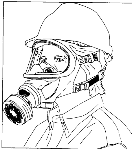
Figure 4-9. Full-facepiece with replaceable, chin-mounted filter.
