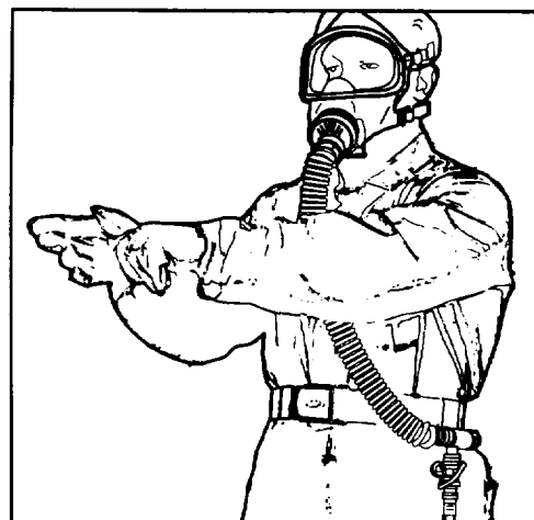
Figure 4-12. Constant-flow supplied-air respirator with a full facepiece.
