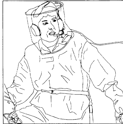
Figure 4-4. Supplied-air hood, long shroud.
