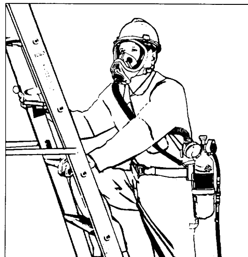
Figure 4-18. Combination pressure-demand airline and short-duration SCBA.
