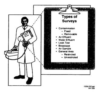
**Figure 8.9 Types of Surveys.** There are many different types of surveys performed by Special Nuclear Material licensees.
