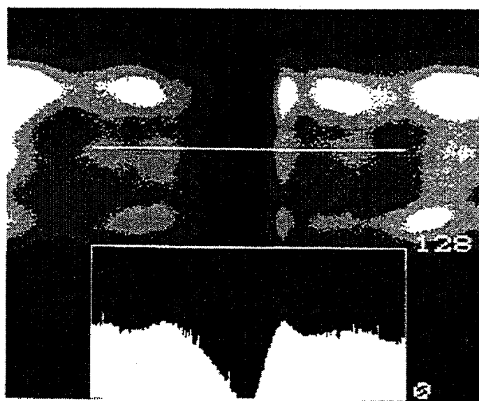
Fig. 4.7. Ultrasonic shadow of a 60% TW laser-cut slot produced by an angled 50-MHz shear wave launched from inside a water-filled tube, which is horizontal in the photograph. Tube axis is represented by the white line. A highly focused (50- \mu\text{m} spot size) water-coupled receiving transducer was used to scan the outer surface of the tube to create the shadow from the through-transmitted ultrasonic waves. Black band is the shadow of the laser-cut slot. Figure below the shadow shows amplitude as a function of position in the shadow along the white line. (Image courtesy of Sonoscan Inc.)
